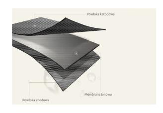
on which hydrogen and oxygen are separated, the hydrogen obtained is pure and of the highest quality.
